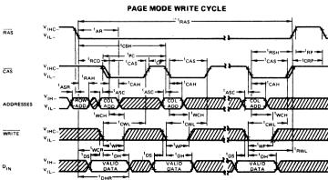
$T_a = 0^{\circ} \text{ to } +70^{\circ}\text{C}; V_{CC} = +5\text{V} \pm 10\%; V_{SS} = 0\text{V}$
